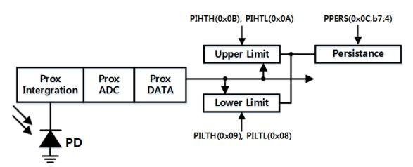
Figure 3. Programmable Interrupt
