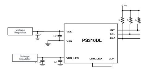
If it is not possible to provide two separate power supplies, the device can be operated from a single supply. A  $22\Omega$  resistor in series with the VDD supply line and a 1-uF low ESR capacitor effectively filter any power supply noise. The previous capacitor placement considerations apply.
